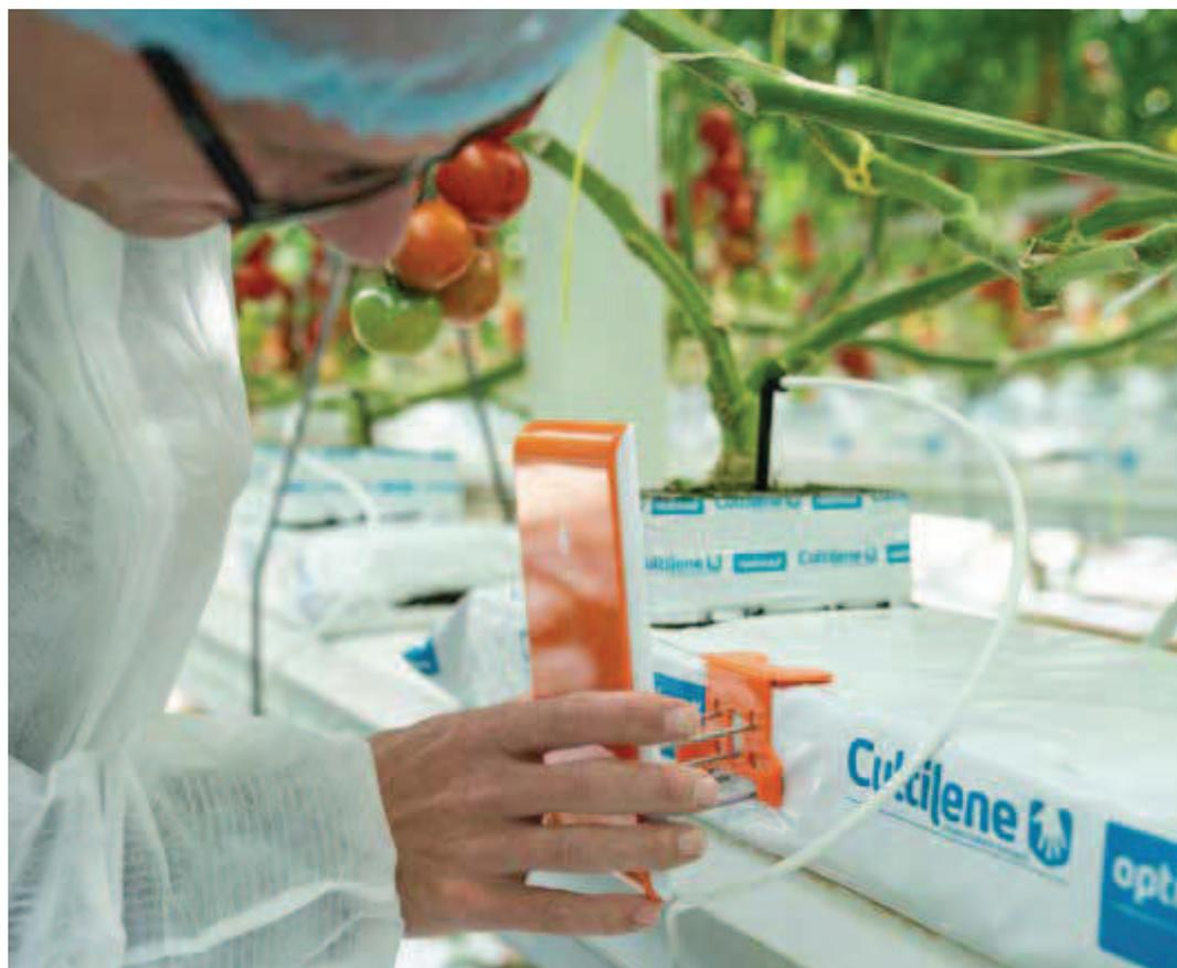
**Each sensor has five pins which are inserted horizontally into the slab.**
