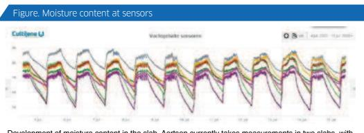
Development of moisture content in the slab. Aertsen currently takes measurements in two slabs, with five sensors per slab. Each line represents one sensor. The irrigation cycles and dry-back in the slab are clearly visible in brief peaks and a prolonged, sharp drop in the water content.
