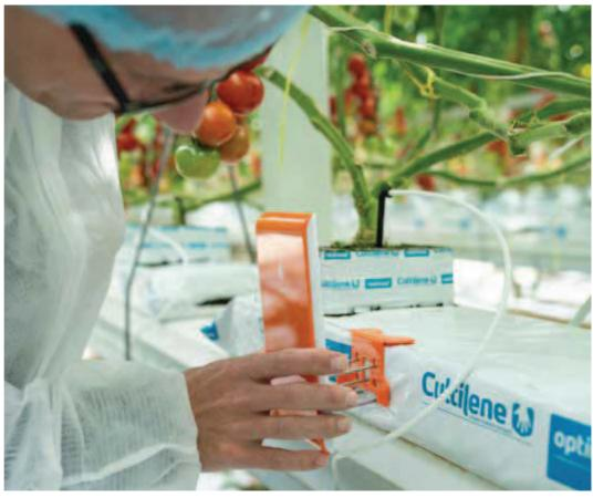
Each sensor has five pins which are inserted horizontally into the slab.
